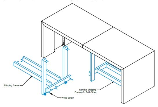
Fig 05: Shipping Frame Removal
