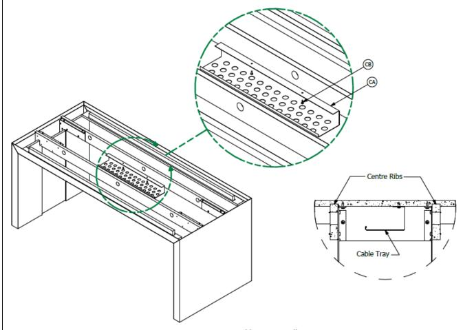
Fig. 12: Cable Tray Install
