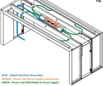
Fig. 14: Undermount USB-A\C 36W Cable Management
